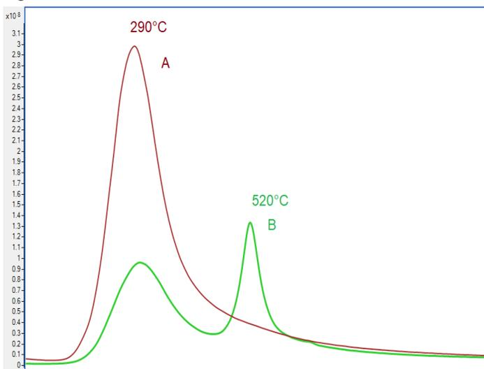
Figure 1. EGA Overlay of 2 Plastic Pyrolysis Oils.
