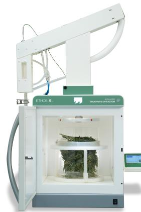
The ETHOS XL has been built for medium-large size producers and has a rotating drum with a total capacity of 45 L and semiautomated workflow for more intense production needs.
