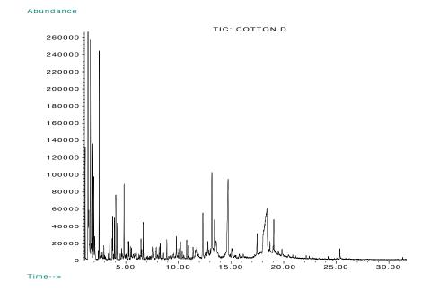
Figure 1. Pyrogram of cotton thread pyrolyzed at 750°C.
