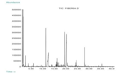
Figure 2. Pyrogram of PET pyrolyzed at 750°C.
