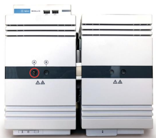
Figure 1B. Three-channel NGA analyzer. The red circle indicates the sample inlet.
