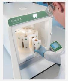
Milestone Ethox X microwave extraction system with SK-12 medium pressure rotor.
