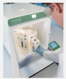
Milestone Ethox X microwave extraction system with SK-12 medium pressure rotor.
