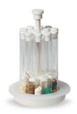
pressure vessels are not needed. Samples are weighed into auto sampler-type vials with the appropriate digestion acid and loaded into a rack.
