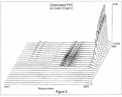
Pyrolysis/FT-IR can be used in the pulsed mode to allow for quick identification of polymer samples as well as in a programmed mode. The programmed mode reveals a time-resolved study of polymers as they degrade. Combining these two modes of operation gives an added dimension to FT-IR analysis of polymers.
