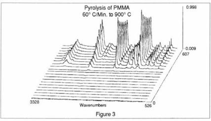
Bands in the fingerprint region are helpful in identifying various compounds. Much like pyrolysis/GC provides a fingerprint for qualitative identification of polymers; direct pyrolysis/FT-IR can be used to give a quick determination of polymer identity.
