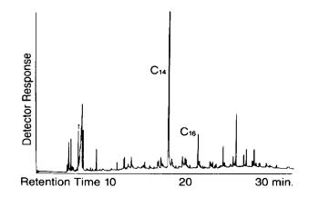
Figure 2. Pyrolysis of Bathroom Cleaner after Headspace Analysis
