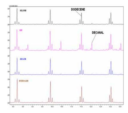
Figure 2. Expanded pyrograms showing aldehydes produced when Polyethylene is pyrolyzed in air.
