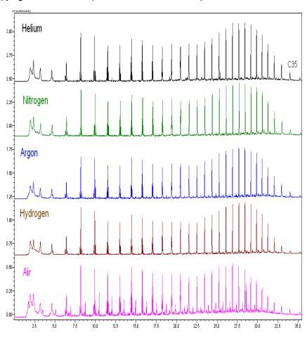
Figure 1. Pyrolysis of Polyethylene in five atmospheres, at 750°C with GC/MS analysis in helium.
